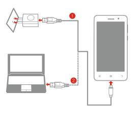
Method 1. Connect your phone to a power outlet using the included cable and USB power adapter.
